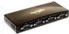
USB To RS-232 Adapter Quad: WK-USB232-4
